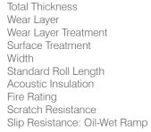
2.00mm 0.70mm HyperGuard+™ Sanitec ™ 2m & 4m 25 l/m Lw 7 dB 7.5kW/m<sup>2</sup> CRF Class T R10
